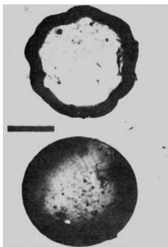
Fig. 2. Photomicrograph of cross-sectioned IPN-modified beads in ethanol. Top: polymer 4 + 25% PU; bottom: polymer 5 + 28% PU; bar represents 0.5 mm. (See also Fig. 12 for release rate data and Fig. 13 for SEM X-ray line scan.)
